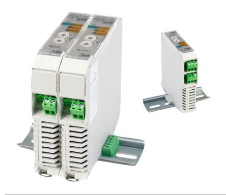
The Loop Drive Booster (LDB) is the heart of the Loopdrive system. This device drive up to 200 FIM's over a dual-core cable. A single LDB can pass 800 W of audio signs from an amplifier and injects at the same time DC to the loop for powering an managing FIM modules. One amplifier channel can be split into multiple LDB i parallel, creating multi-loop with individual surveillance for multi-zone pagin applications.
